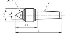
Live centers are for clamping heavy workpiece in lathe. Rigid structure and placing revolving part is characterized long working life. Live centers with accuracy EXTRA is used on grinding machine. Live centers are supplied with apex angle 60° and 90°. Shanks of live centers correspond to standard DIN 228 and ISO 296 without clamping thread. Protection of bearing from the ingress of coolant, dirt or swarf is provided by the built-in ring gasket which also prevent loss of lubricant.
